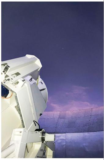
One of the Simons Observatory's small-aperture telescopes looks up at Jupiter in the night sky as part of the calibration process. *Credit*: Allen Foster
